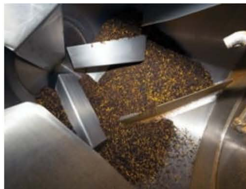
🔥 The Rotary Batch Mini Mixer's tumble-turn-cut-fold action achieves uniformity in three minutes with no product degradation, according to Munson Machinery. (Image courtesy of Munson Machinery)
