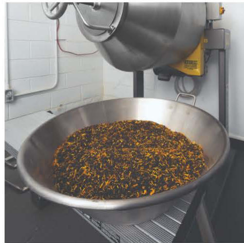
🔥 Biron Teas' 3-cubic-foot (85 l) capacity Rotary Batch Mini Mixer blends teas with or without liquid additions in three minutes with no shear or damage to delicate ingredients, Munson Machinery says. (Image courtesy of Munson Machinery)
